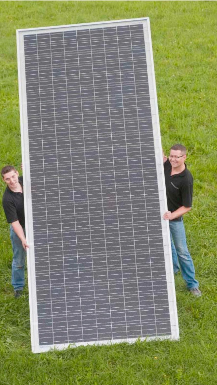
One of the world's largest lightweight solar modules with a cover sheet made of PLEXIGLAS® Solar. The module measures approx. 1.6 by 4 meters and has electric power of about 880 Wp.
