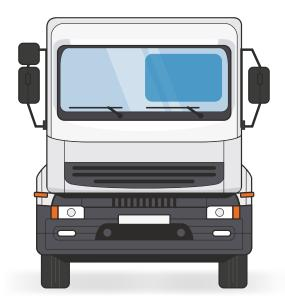
Damage outside of this field of vision (such as chips caused by stones) can also result in rejection if larger than  $a \in 2$  coin or involving cracks that could not be described as minimal (see illustration):
